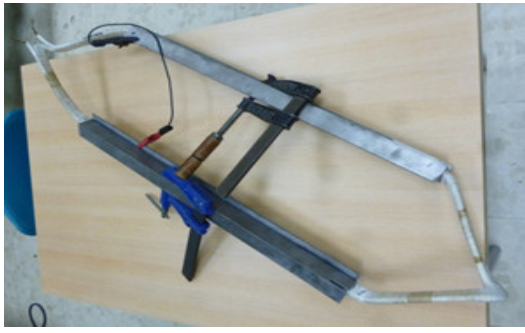
Fig. 4. Complete Stator-Core arrangement using metallic profiles and connecting both sides with a cable
