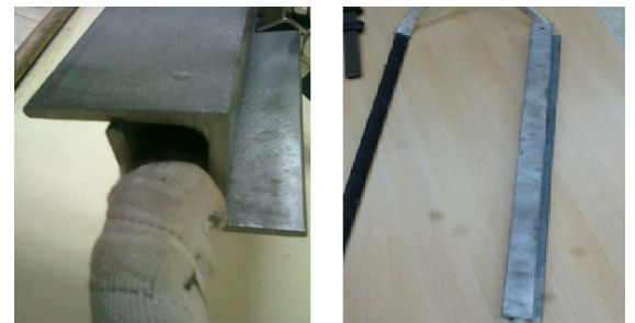
Fig. 3. High conductivity "L" shaped steel profiles arrangement detail for Stator Core simulation for simulating the stator core for the coil
