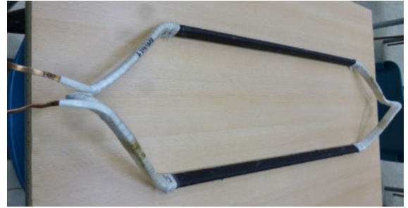
Fig. 2. Stator-Winding Coil under test
